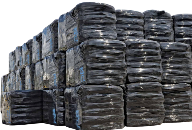
Example of wrapped PEF bales to be produced. These will be transported in sealed shipping containers and transported to markets.
